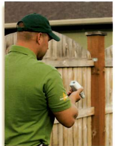
Determine best sensor location using signal strength indicator
